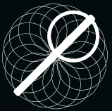
Satellite spray arm coverage
